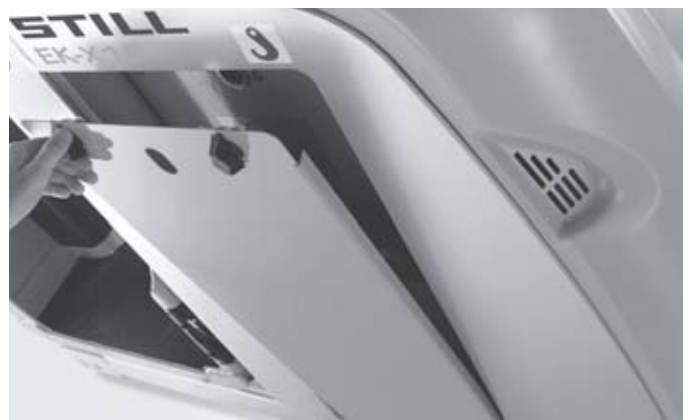
Battery compartment cover can be opened and closed without tools
