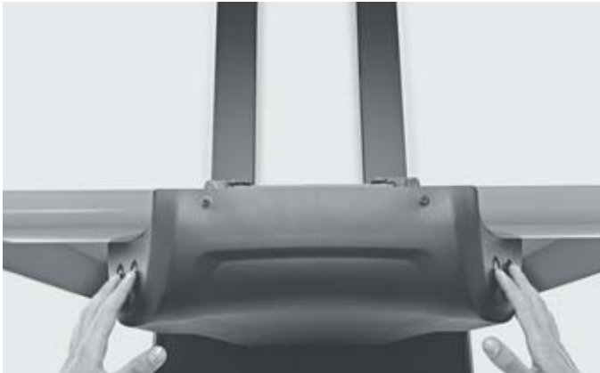
Safe two-hand operation of the auxiliary lift
